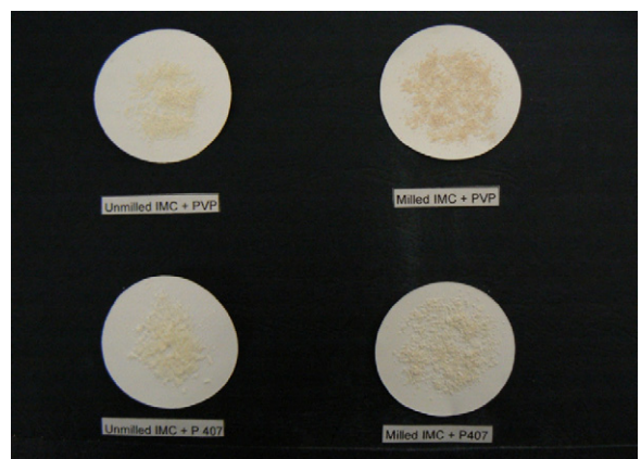
Fig. 4. IMC milled with PVP showed change in colour (white to yellow) after high pressure homogenization. With P407, intensity of yellow colour was less compared with PVP.
